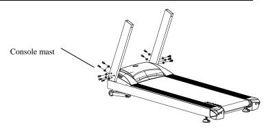
A;)put the console wire through the console mast .
